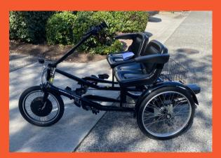
Worksman Side by Side The Side by Side is perfect for those riders that are able to assist with pedaling. It has a comfortable captain's seat with a seat belt, three gears, and adaptive pedals.
