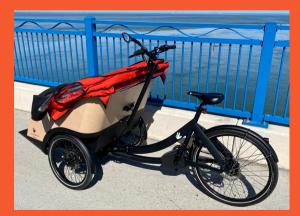
Triobike Taxi The triobike taxi from Denmark can comfortably transport two adult passengers and has a removable footplate for ease of entry and seat belts for added safety.
